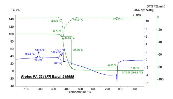
Change in test atmosphere from N₂ to air at 770°C.
